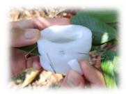
7. Pull off plug to access cage interior. Available for H-type clip cages only.
